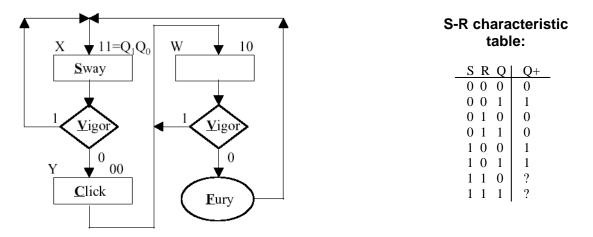
(b) Finish the implementation of the ASM by determining the <u>minimum sum-of-products</u> (MSOP) logic expressions for all the output signals: (8%)
