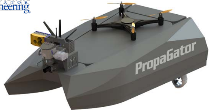
PropaGator 2: UF's Autonomous Surface Vehicle (Robot Boat with quadcopter) for RoboBoat competition
