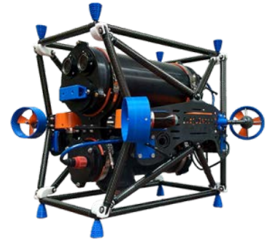
SubjuGator 8 CAD image for the 2016 RoboSub Competition.
