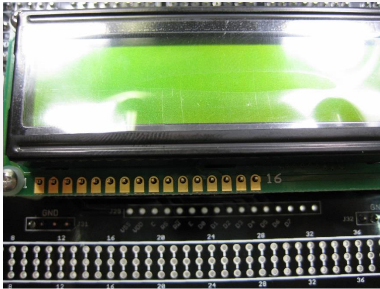
LCD mounted mechanically as viewed from above. Notice the LCD header pins poke through the LCD's board connections.
