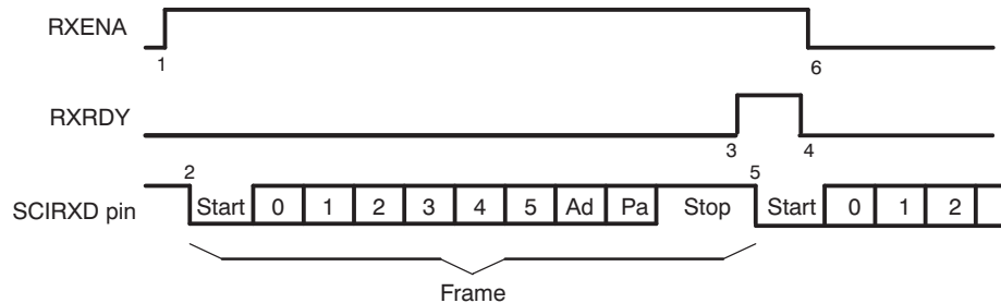
Figure 1-8. SCI RX Signals in Communication Modes
