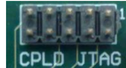
CPLD JTAG for programming an Altera EPM3064ALC44-10 CPLD if populated
