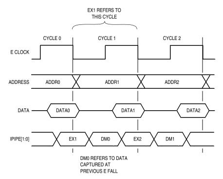
Figure 8-6. Queue Status Signal Timing (M68HC12)
