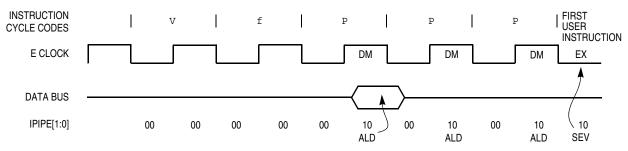
Figure 8-7. Reset Sequence for HCS12
