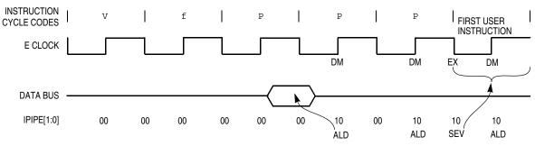
Figure 8-8. Reset Sequence for M68HC12
