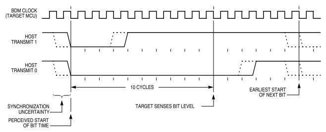
Figure 8-1. BDM Host to Target Serial Bit Timing
