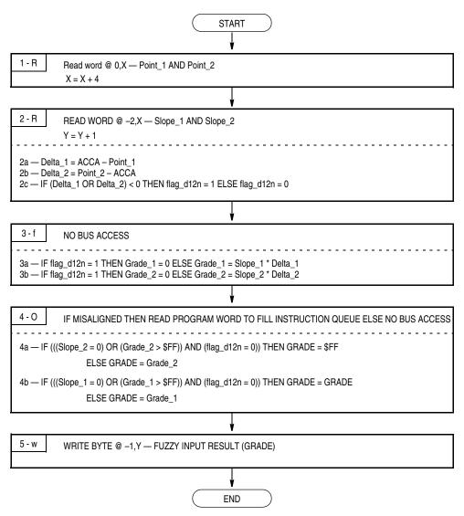
Figure 9-5. MEM Instruction Flow Diagram
