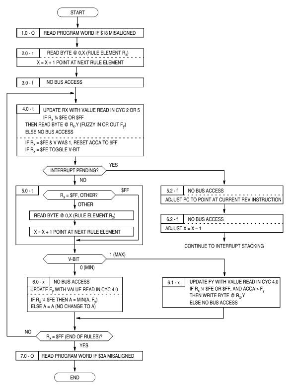
Figure 9-9. REV Instruction Flow Diagram
