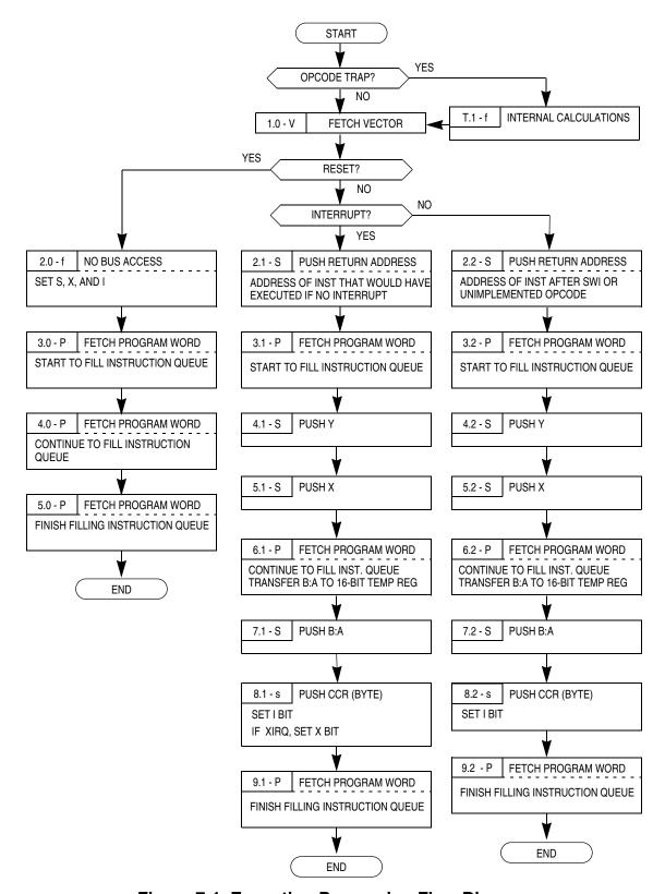
Figure 7-1. Exception Processing Flow Diagram
