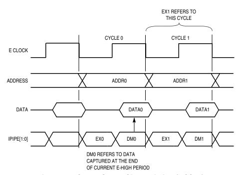
Figure 8-5. Queue Status Signal Timing (HCS12)
