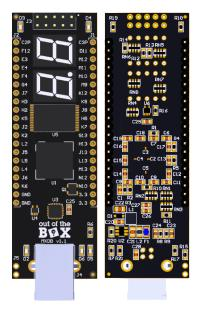
The MXDB is Out of the Box's 2<sup>nd</sup> generation programmable logic development platform. The MXDB is a platform designed specifically for learning the basics of digital electronics from the lowest level of logic gates to microprocessors. The board features a USB FIFO bridge, external flash memory and accompaniment software to program data to the flash memory with a PC. The board's form-factor also makes it ideal for interfacing with a solderless breadboard.
