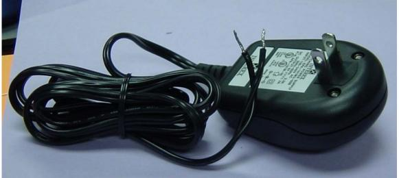
Plug in your supply and measure the ends with your multimeter. Mark the positive end. Place the positive end into the red binding post with a red jumper wire. Place the negative end into the black binding post with a red jumper wire as shown below.
