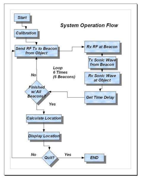
Next, the geometry involved in the position calculation must be specified completely for the processor. Even after all of the above challenges have been successfully addressed we will be left with a list of distances from the receive unit to each of the remote beacons in the room. These distances, together with the
