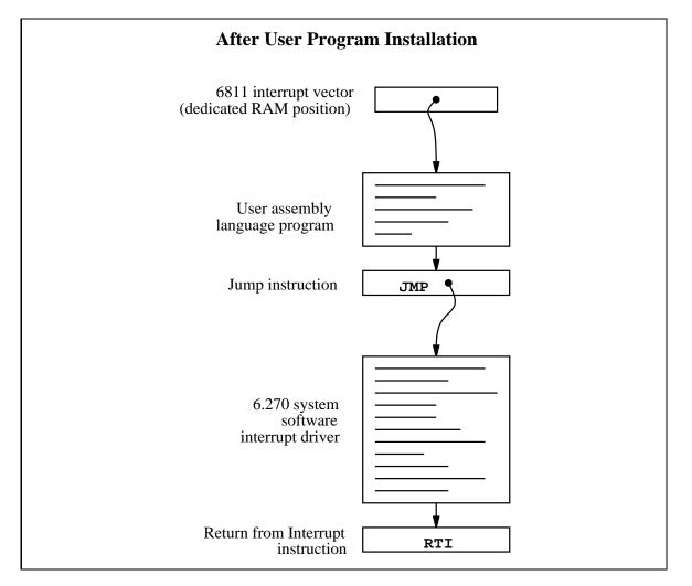
Figure 6.5: Interrupt Structure After User Program Installation
