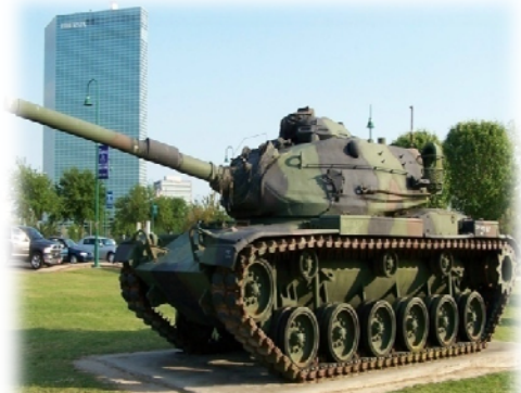
Figure 6: M60 Patton, example of continuous track
