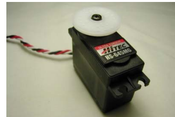
Figure 7: HS-645 High Torque Servo
