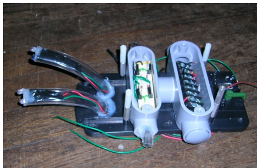
Figure 5: Conduit boxes above main chassis
