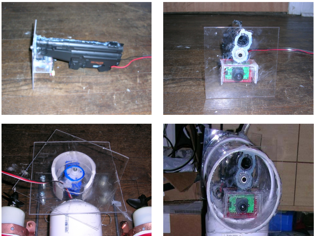
Figure 13: (a) top left is the airsoft gun with the camera attached below it (b) top right is the camera attached below the gun from the front (c) bottom left is the servo mount for the camera housing (d) bottom right is the camera housing itself fully sealed and ready to go.
