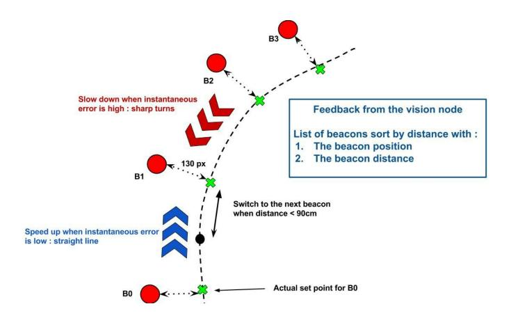
Using the detected beacons list it gets from the image processing node, the first role of the master node is to define a setpoint and to make sure that Carver will reach it.
