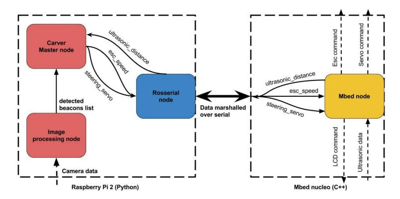
The raspberry Pi hosts the three high level processing nodes:
