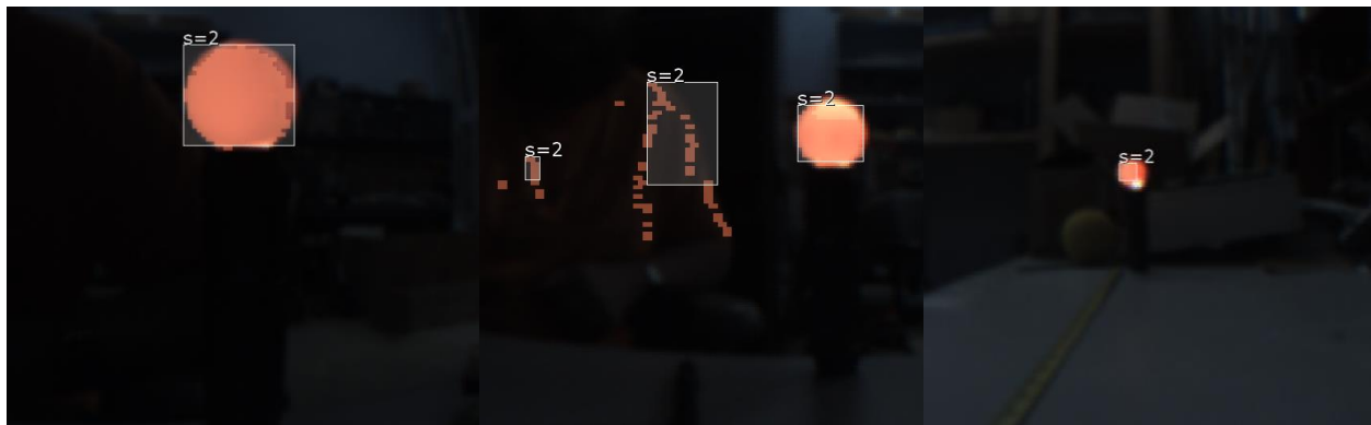
Figure 12 shows the tracking of the orange ping pong at distances 7, 13, 30 inches respectively. You can see the camera picking up spots from my neon orange shirt in the middle image.
