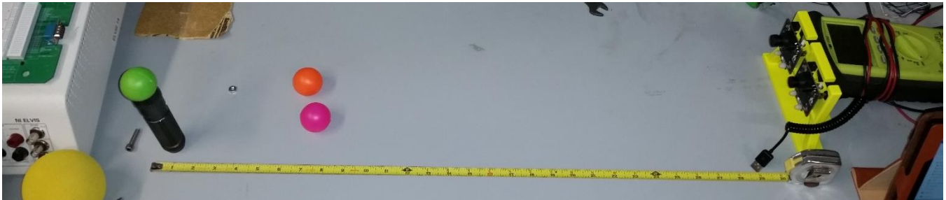
Figure 11 shows my experimental setup for this test. On the left you can see the flashlight with a green ping pong resting on top of it. To the right in the yellow stand is the Pixy camera used for this test. I used a brightness of 25.
