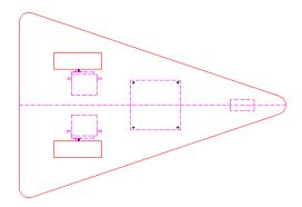
automobile. The second and final design makes use of mechanics present in cars today. An approximate Ackerman's steering model is used. Ackerman's theory uses geometry to describe a system in which the inner wheel during a turn turns tighter then the outer
