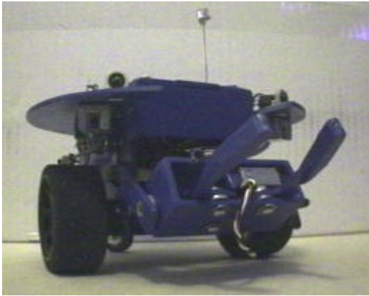
Fig. 2 & 3, Smurf viewed from the front. The microphone sensor can be seen at the top of the images. This was an initial stage where only two IR detector/emitter pairs are mounted.
