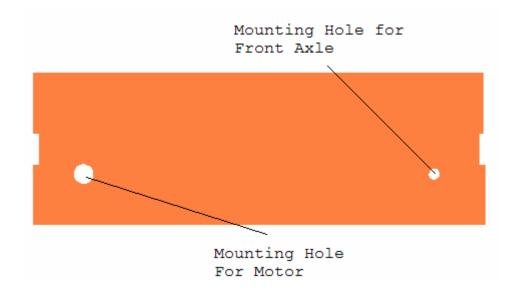
The bottom of SEAL's body consists of a 9x5 piece of wood that has been glued to the four side pieces.
