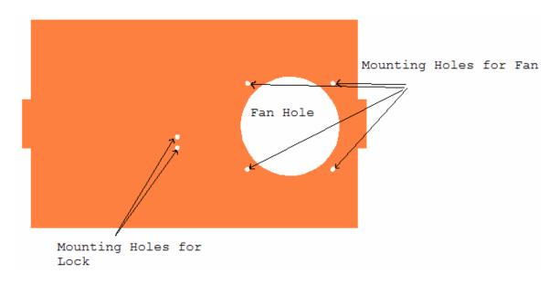
The back of the robot is the same size as the front. Instead of fan and lock mounting holes, it has for holes in the bottom to help the air brought in by the fan in front to circulate throughout the robot and exit in the back. The following is a figure showing the design of this piece.
