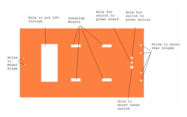
The final piece of SEAL's platform is the pendulum. The main pendulum mounts are constructed using four pieces of wood. Two of the pieces are then glued together to form one mount and likewise for the other two. An example of the pendulum mounts can be seen below.
