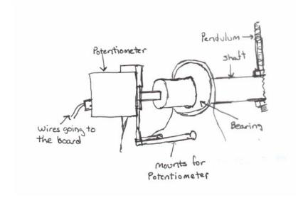
When attached in this manor, the potentiometer is able to sense the position of the pendulum as the ball falls forward or backwards. The bearing provides the shaft with the ability to move smoothly, and the mounts for the potentiometer stop the potentiometer from moving when the pendulum rotates.
