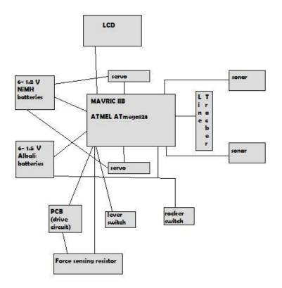
GIR's microcontroller is the ATMEL ATmega128 on a MAVRIC IIB board. The electrical components of GIR include the following:
