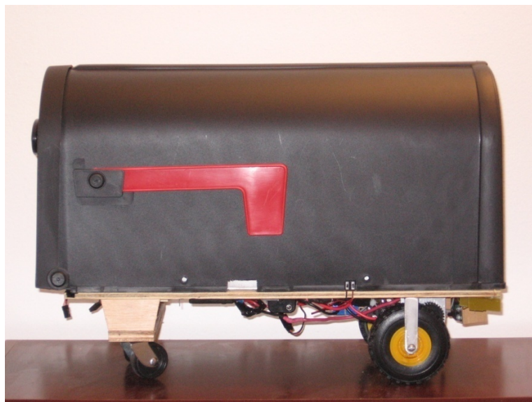
Figure 2. The assembled mobile robotic platform
