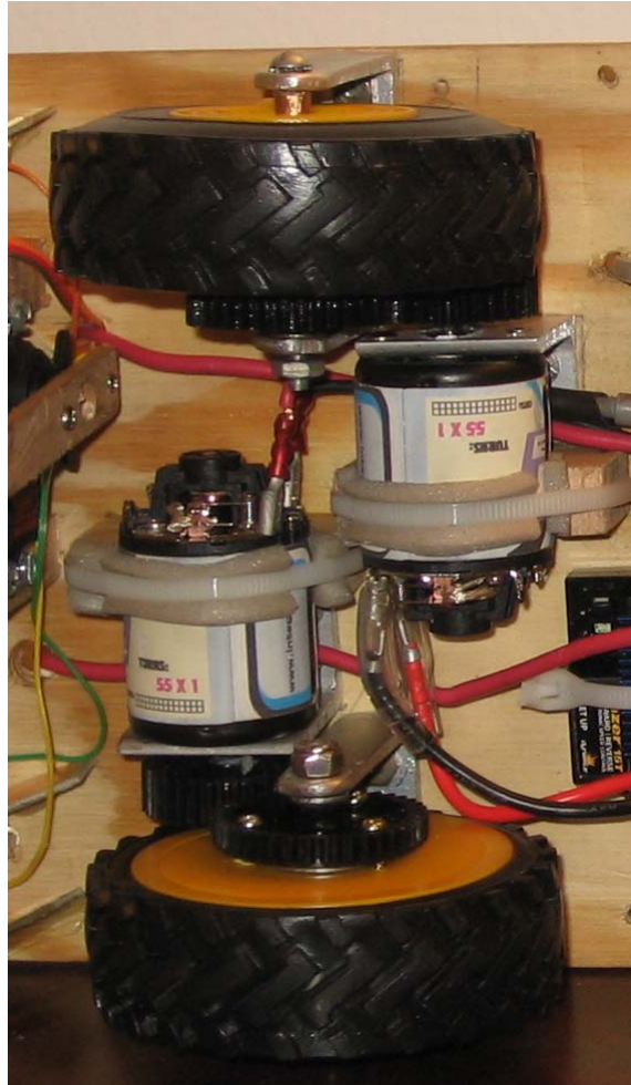
Figure 12. The Integy 55t motors attached to the rear drive wheels
