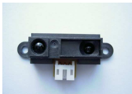
Figure 8. Sharp GP2D12 infrared sensor.
