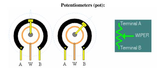
Potentiometer Resistance =  $R_{AB}$   $R_{AB} = R_{AW} + R_{WB}$
