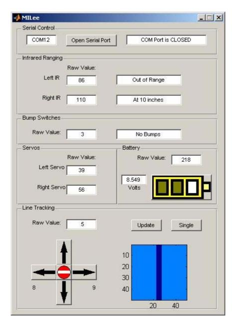
An additional sort of sensor is the batter level monitor. This simply divides the 9V battery voltage in half, and then converts it to a digital value to allow for the robot or user to know the current status of the battery life (through either internal software behavior, the onboard LED, or through the GUI) and when it will need to be changed.
