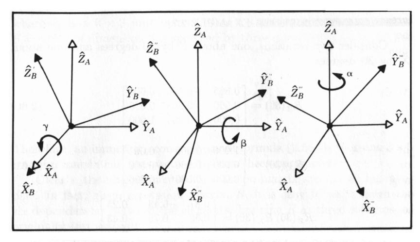
Start with the frame coincident with a known reference frame  $\{A\}$ . First rotate  $\{B\}$  about  $\hat{X}_A$  by an angle  $\gamma$ , then rotate about  $\hat{Y}_A$  by an angle  $\beta$ , and then rotate about  $\hat{Z}_A$  by an angle  $\alpha$ .
