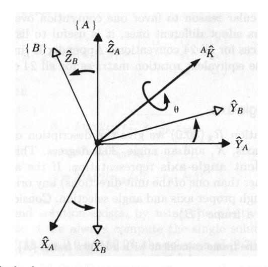
Start with the frame coincident with a known frame  $\{A\}$ . Then rotate  $\{B\}$  about the vector  ${}^{A}\hat{K}$  by an angle  $\theta$  according to the right-hand rule.
