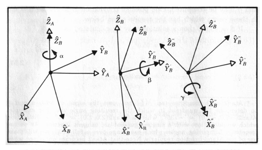
Start with the frame coincident with a known frame  $\{A\}$ . First rotate  $\{B\}$  about  $\hat{Z}_B$  by an angle  $\alpha$ , then rotate about  $\hat{Y}_B$  by an angle  $\beta$ , and then rotate about  $\hat{X}_B$  by an angle  $\gamma$ .
