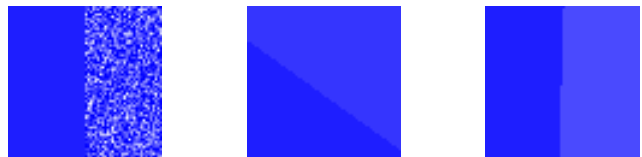
Fig. 1. The wedgelet transform fails to detect the edge correctly: (left) original image, (center) wedgelet, (right) MLDA atom
