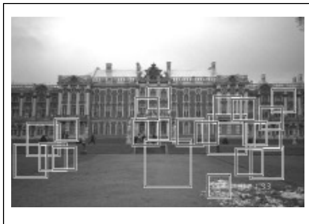
Figure 4: Some false detections obtained with the first version of the system. This false positives were later used as non-face examples in the training process
