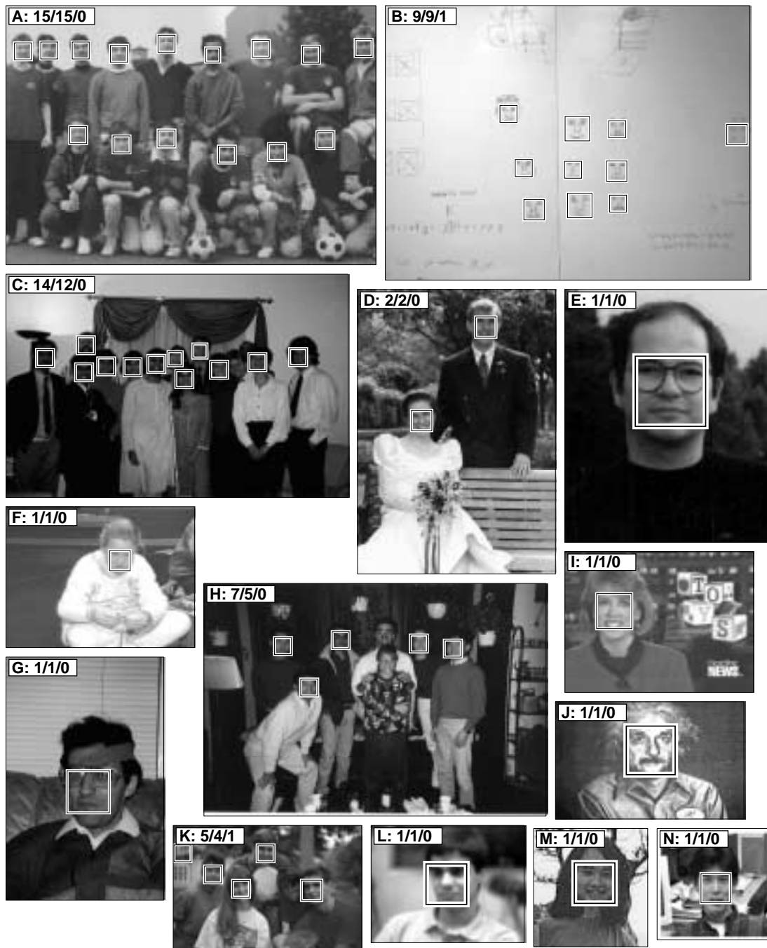
Figure 12: Output obtained in the same manner as the examples in Fig. 11. Some notes on specific images: Faces are missed in C (one due to occlusion, one due to large angle), H (reflections off of glasses made the eyes appear brighter than the rest of the face), and K (due to large angle). False detections are present in B and K. Although the system was trained only on real faces, hand drawn faces are detected in B. A, B, J, K, and L were provided by Sung and Poggio at MIT, C, D, E, G, H, and M were scanned from photographs, F and I are digitized television images, and N is a CCD image.
