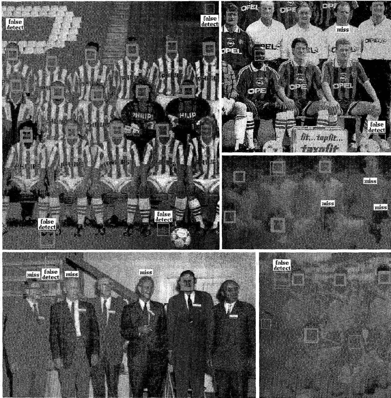
Fig. 7. Some face-detection results with mistakes. The top right image is very heavily quantized with only 46 gray levels. The system misses only one face. In the middle right image, the system misses some faces with significant illumination shadows. In the bottom left image, the system misses some faces with fairly large rotation components. Most of the false detects are images patches with eye-like dark regions. Note: The images here are not among those from our test databases.
