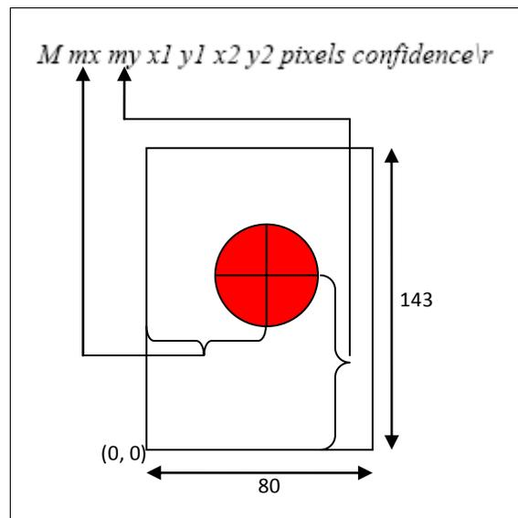
Figure-7: Data packet returned by CMUcam TC command
