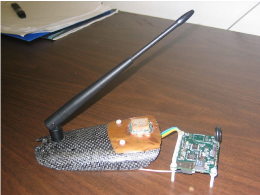
Figure 2: Revision 5 Onboard Electronics
