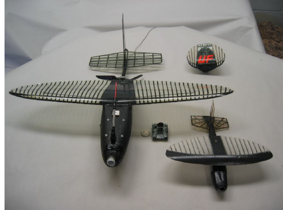
Figure 4: 4", 10", and 24" MAVs with the Onboard System Vehicles," SAMPE Journal , vol. 37, No. 4, pp. 7-13, July/August 2001.
