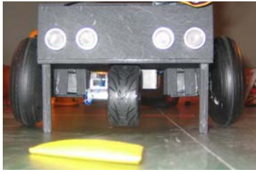
Figure 3. Docked hitting wheel in center of the platform.
