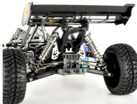
Figure 4. The XTM Rail spoiler and rear shocks. The motor controller can be seen on the right.
