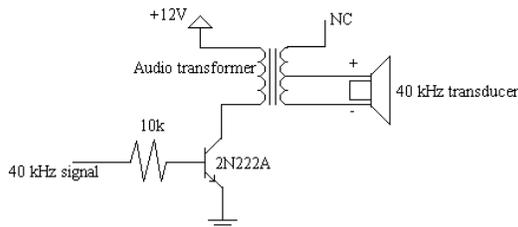
Figure 1: Sonar Transmitter
