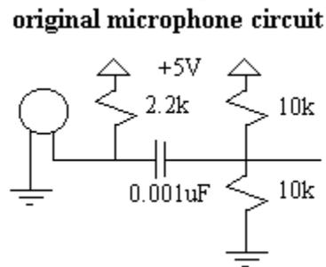
By replacing the 0.001 uF capacitor with a 0.1 uF capacitor, the range was increased to approximately two inches. However, increasing the capacitor value to 1 uF and 10 uF had no further effect on the range.
