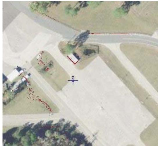
Figure 5. Scan points (red) overlaid on a satellite image of the test area. The vehicle position is shown by the gray box and blue lines.
