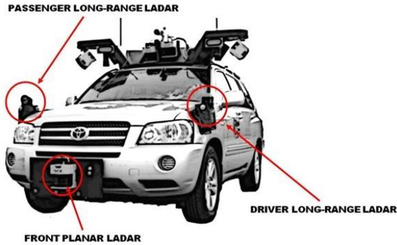
Figure 2. The position of the LRFs used for testing (marked as Passenger and Driver Long-Range LADAR).
