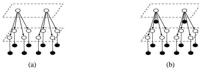
Fig. 1. Differences in TSBN models: (a) observable variables at the lowest layer only; (b) our approach: observable variables at all layers. Black nodes denote observable variables and white nodes represent hidden random variables connected in a tree structure.
