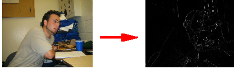
Figure 3–1: The absolute value of the output of the Sobel gradient module emphasizes the edges in the previous image.
