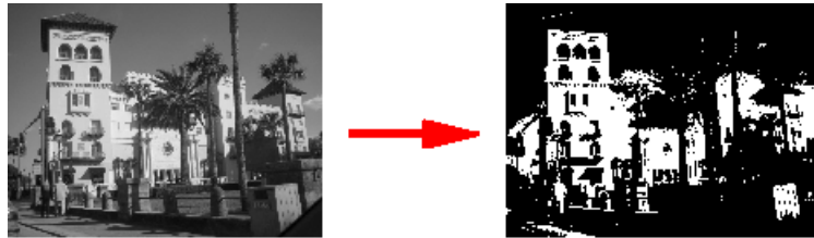
Figure 3–2: The output of the threshold module is a binary (Two color) image.
