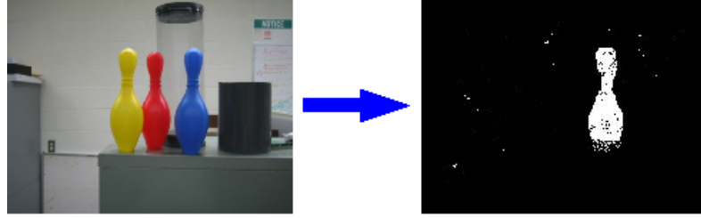
Figure 4–2: The bandpass threshold module produces a binary image that represents the two classes of data (blue bowling pin and not a blue bowling pin)
