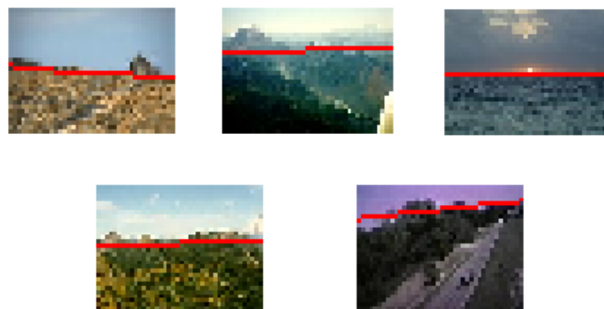
Figure 4–6: The horizon line is approximated for several test images. Performance of the algorithm can be increased or decreased based on the number of possible horizons tested.
