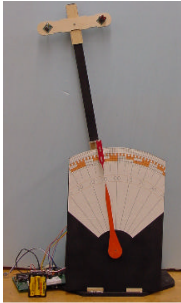
Figure 3-5: Dynamic Inclinerometer Test Platform
